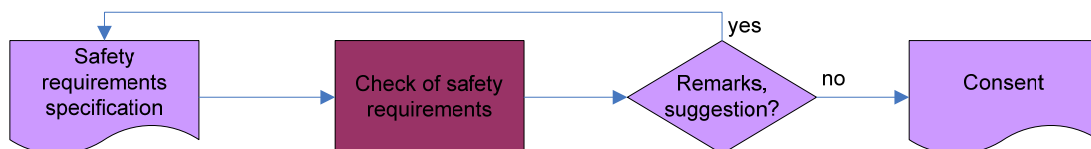
Figure 15 – Check of safety requirements
